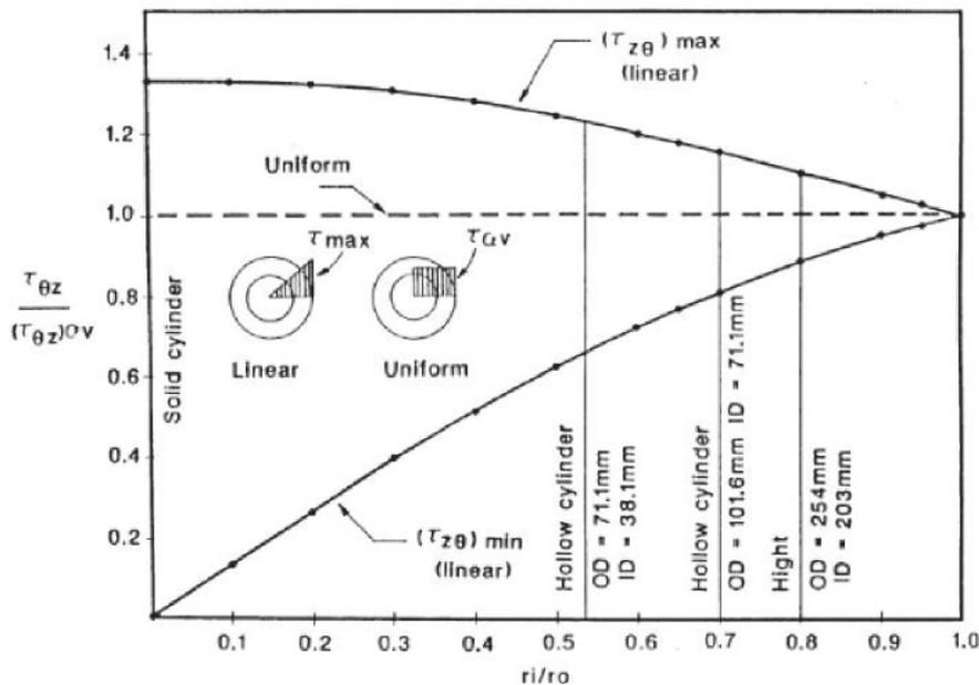
**Figure 9** : Shear stress distribution in a hollow Torsional shear specimen (Porovic, 1995)
