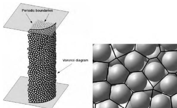
**Figure 4** : DEM specimen in the simulation and subplot of Voronoi diagram ( Cui et al.,2007)
