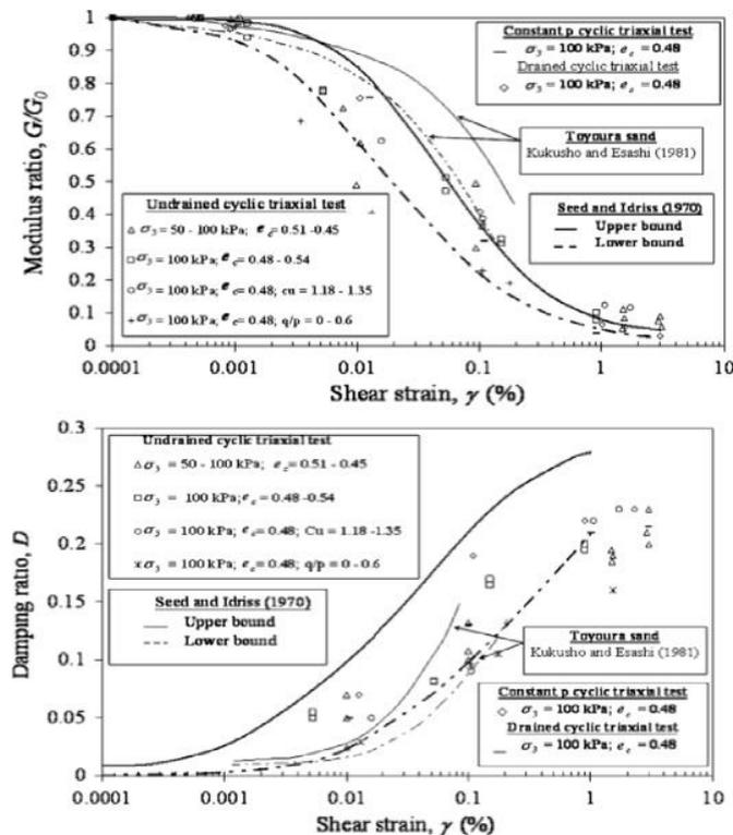
**Figure 12:** Comparison of shear modulus and damping ratio obtained and numerical tests with standard curves (Sitharam and Vinod, 2010)
