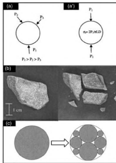
**Figure 7 :** Idealization of induced tensile stress, and fragments produced after tensile failure of real aggregate and idealized material (Lobo-Guerrero and Vallejo, 2005)
