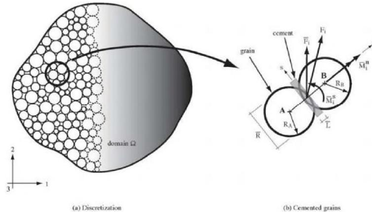
**Figure 2** : Particulate DEM model (Bobet, 2009)
