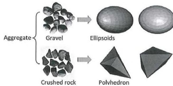
**Figure 6 :** Representation of gravel and crushed rock by ellipsoids and polyhedrons (He et al., 2012)
