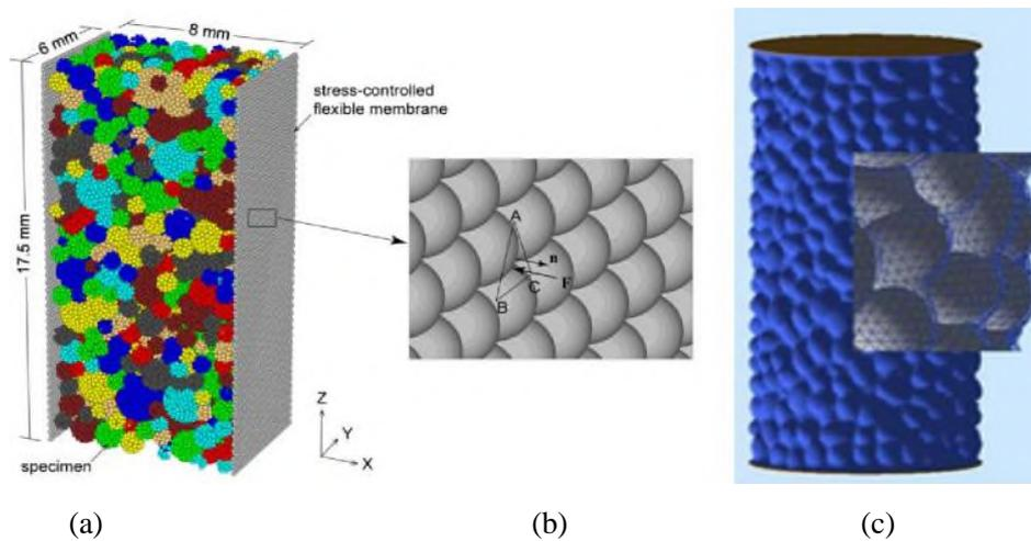
**Figure 5:** Flexible boundary adopted by Wang and Yan (2011b) (a) typical specimen comprising of crushable agglomerates; (b) equivalent force applied on a unit particle triangle (c) DEM GTSC simulation the triangular lattice membrane (Knuth et al., 2012)
