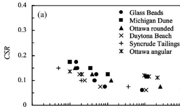
**Figure 10 :** Liquefaction susceptibility for different simulated soil samples (Ashmawy et al., 2003)
