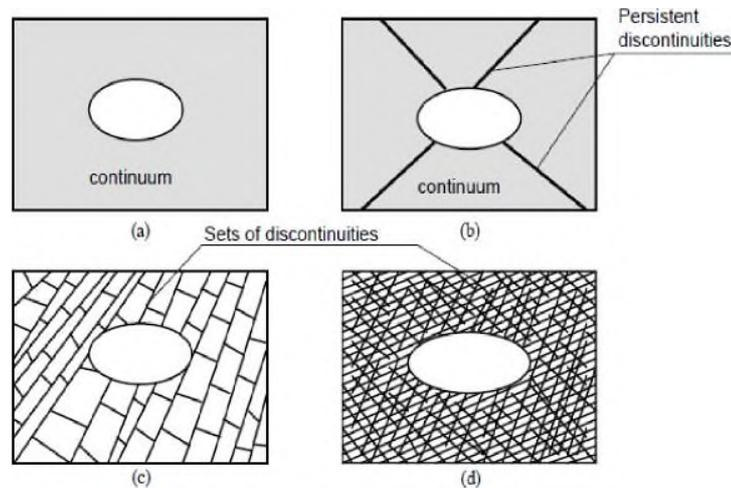
**Figure 1:** Selection of different numerical methods (a) continuum method, (b) continuum with fracture element or discrete method, (c) discrete model and (d) continuum method with equivalent properties (Jing, 2003)
