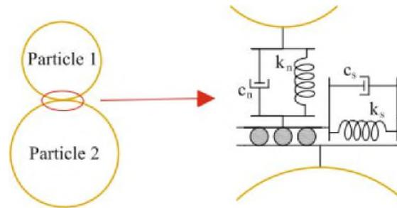
**Figure 3:** Schematic of the constitutive law of normal and shear contact forces between two particles (Zamani and El Shamy, 2011)
