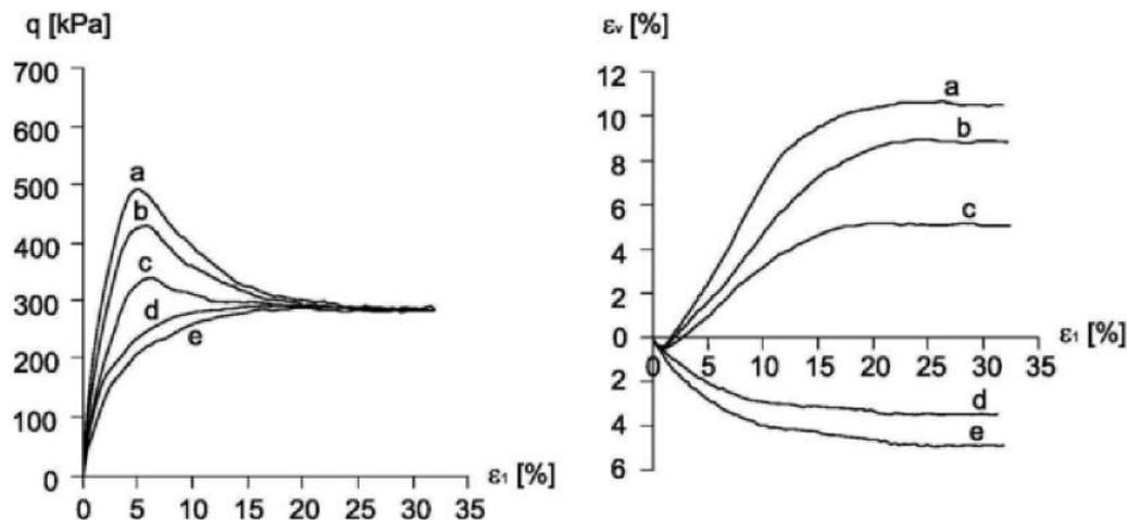
**Figure 11:** Discrete simulations of triaxial test for granular specimen: global deviatoric stress and volumetric strain versus axial strain for different initial void ratio  $e_0$ : a)  $e_0 = 0.50$ , b)  $e_0 = 0.60$ , c)  $e_0 = 0.70$ , d)  $e_0 = 0.80$ , e)  $e_0 = 0.90$  ( $E_c = 30$  GPa,  $\nu_c = 0.3$ ,  $\mu = 30^\circ$ ,  $\beta = 0.15$ ,  $\eta = 1.0$ ,  $p = 100$  kPa,  $d_{50} = 5$  mm) (Widulinski et al., 2009)
