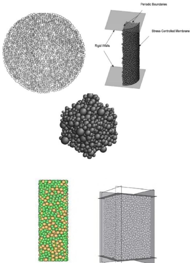
**Figure 8:** Biaxial and Triaxial samples generated by Sitharam (2003), O’Sullivan et al., (2008), Sitharam and Vinod (2010), Anitha and Sitharam (2010) and Nguyen et al., (2014).
