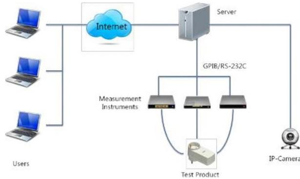
Fig. 1. System configuration.
