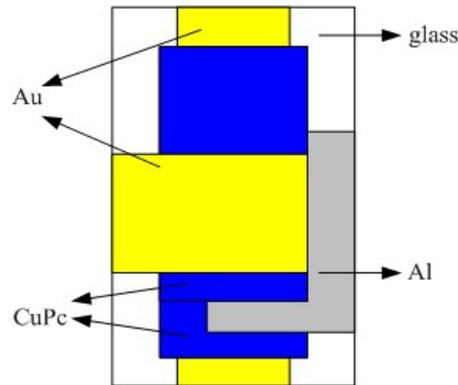
Fig. 1. The OSIT structure diagram
