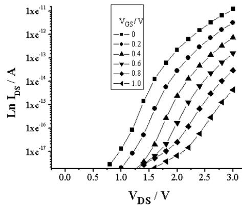
Fig. 3. The I-V characteristic curves of OSIT in semi-log coordinate
