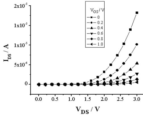
Fig. 2. The I-V characteristic curves of OSIT
