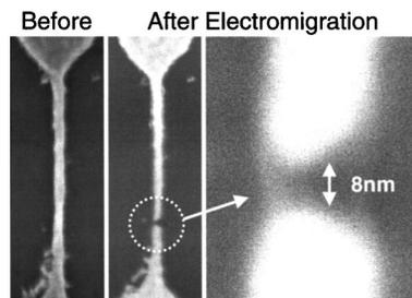
FIG. 5. 20 nm gold nanowire before and after the electromigration process conducted at 175 °C. The gap between contacts is approximately 8 nm.
