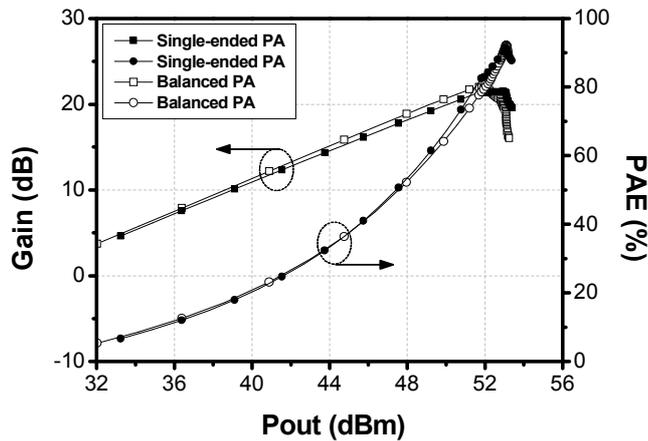
Fig. 4. Simulated results: gain and PAE.
