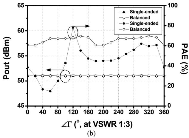
Fig. 5. Simulated output power and PAE of the single-ended and balanced class-E amplifiers under the load mismatch condition of 1:3 VSWR: (a) fixed input power to have an output power of 53 dBm at the 50  $\Omega$  load, (b) fixed output power of 51 dBm.
