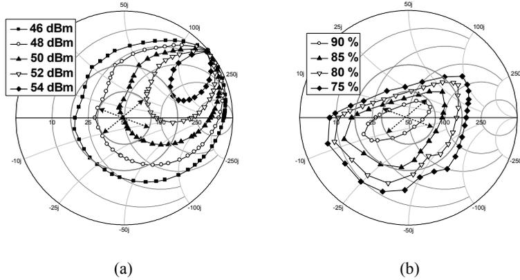
Fig. 2. Load-pull simulation results for the single-ended class-E amplifier: (a) output power, (b) efficiency.
