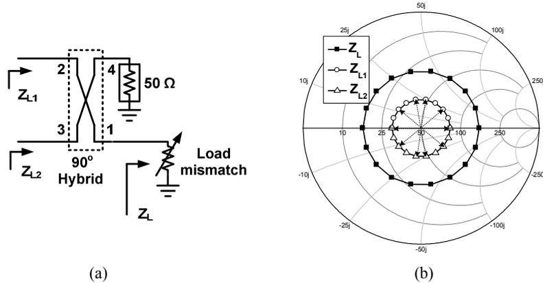
Fig. 1. (a) load network with a  $90^\circ$  hybrid coupler, (b) impedances for the mismatch condition for a VSWR of 1:3.
