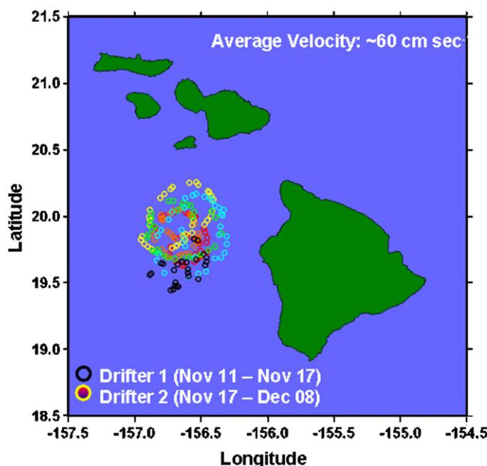
**Fig. 14.** ARGOS positions of the surface temperature-string *Drifter 1* (black circles) and the METOCAN bio-optical *Drifter 2* (colored circles) during E-Flux I. Results suggest that both surface drifters made multiple revolutions around the eddy's center as it slowly moved north after the shipboard survey.
