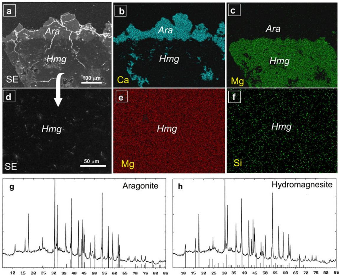
**Fig. 11** **a** SEM image of subsurficial cross section of living cyanobacterial mat taken from c. 4 m water depth (sample A-48). The topmost part of the section is composed of aragonite (*Ara*) passing downward into hydromagnesite (*Hmg*). **b**, **c** EDS maps for Ca
