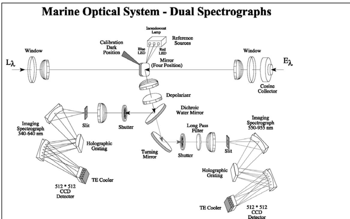
Figure 2.8: A schematic diagram showing the optical design of the MOS spectrographs.
