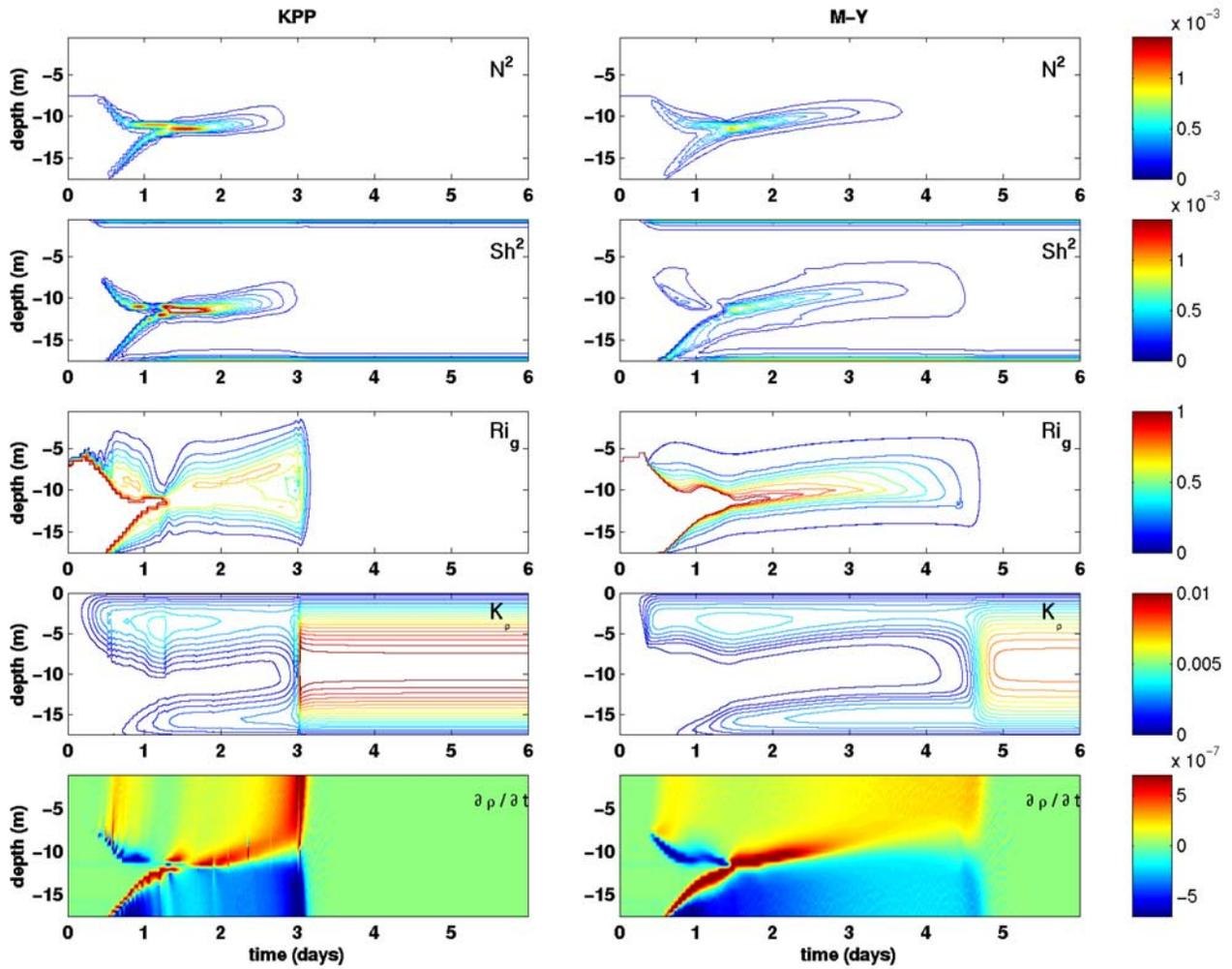
**Figure 16.** Time-depth contour plots of various fields associated with vertical mixing  $N^2$ ,  $Sh^2$ ,  $Ri_g$ ,  $K_p$ , and  $\partial\rho/\partial t$  for the  $N_o/10$  interacting boundary layers experiment.
