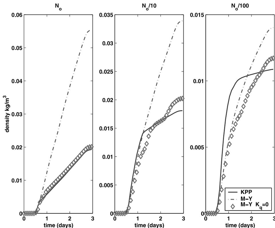
**Figure 9.** Time series of change in surface density with three different initial stratifications for simulations with the two mixing schemes and for the M-Y scheme with the vertical diffusion of turbulent kinetic energy and length scale excluded.
