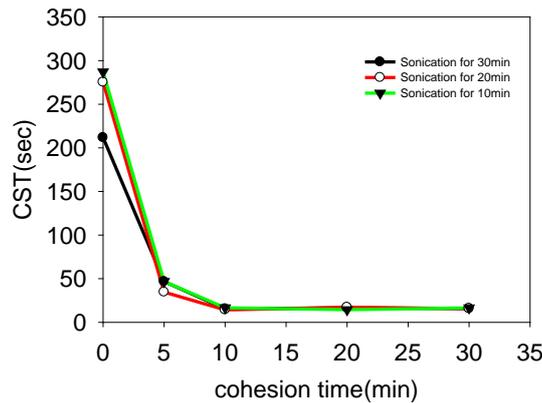
Fig. 3. CST with Ultrasonic Treatment
