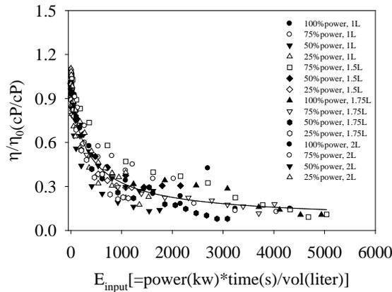
**Fig. 1.** Viscosity Reduction with Input Energy
