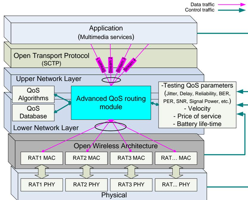
**Figure 1. Advanced Mobile Equipment with Incorporated Advanced QoS Routing Algorithm**
