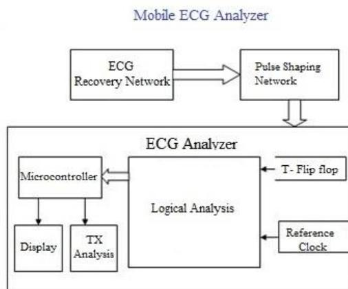
**Figure 3. Essential blocks of ECG analyzer**
