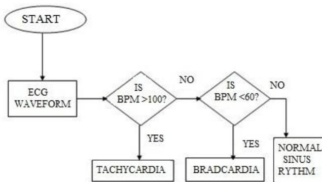
**Figure 4. Flowchart showing the logic of ECG analysis**
