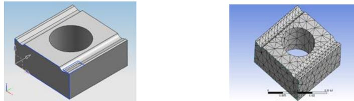
Figure 8. Chart, Meshing of Cutting Tool Model
