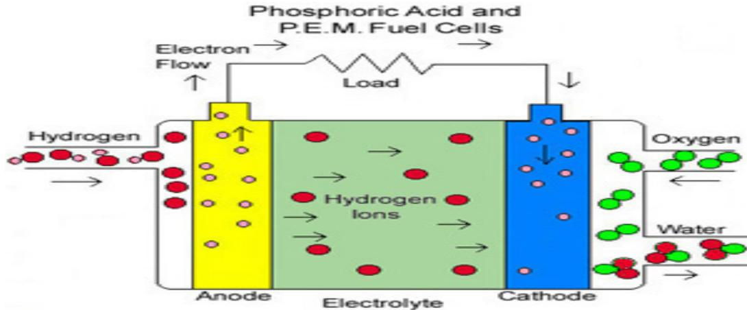
**Figure 4. Basic Hydrogen Fuel Cell System [7]**
