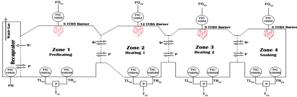
**Figure 1. Structure of a Walking Beam Reheating Furnace.**
