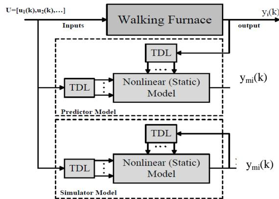
**Figure 4. General Structures of Simulator and Predictor Models.**
