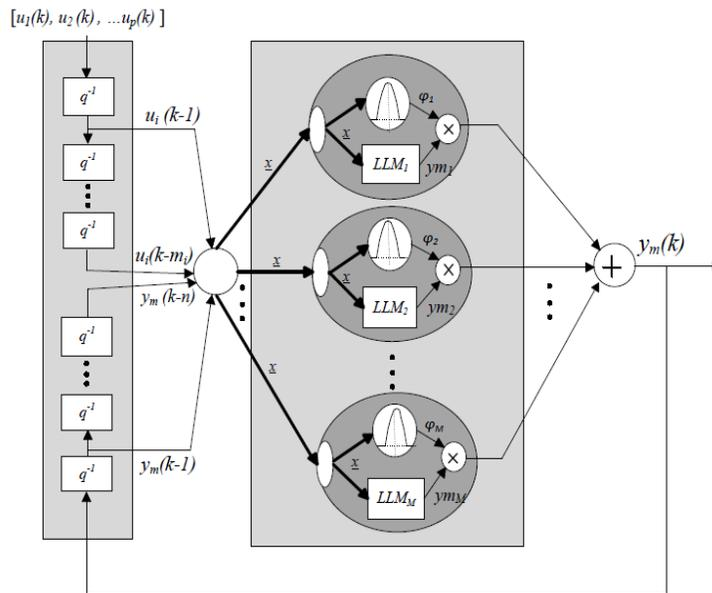
**Figure 5. Architecture of Recurrent Local Linear Neuro-fuzzy Network**
