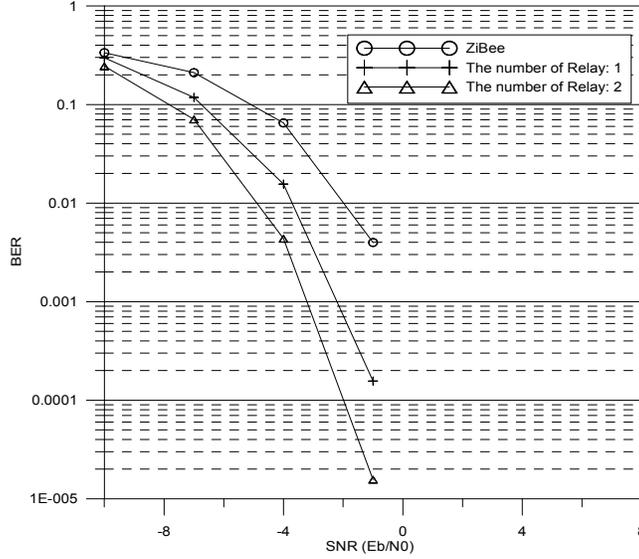
**Fig. 1.** BER performance comparison of the number of relay based on ZigBee.
