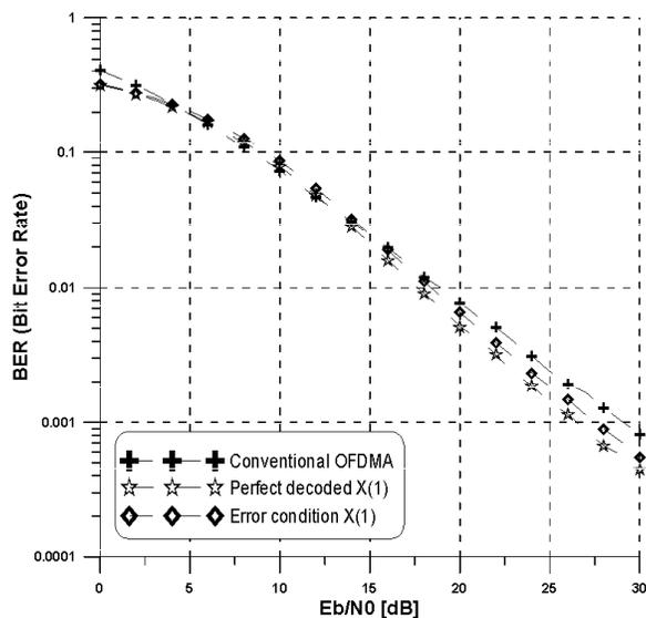
**Fig. 1.** BER performance of proposed scheme compared with OFDMA system according to relative condition of inter-user channel (3[dB]) and error condition of  $X(1)$ .
