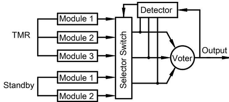
**Figure 1. Architecture of the Hybrid Redundancy System**
