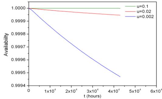
**Figure 9. Effects of Repair Rate on the Availability of the System**
