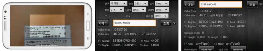
(b) cable installation-support service (barcode scanning, detailed cable information)
