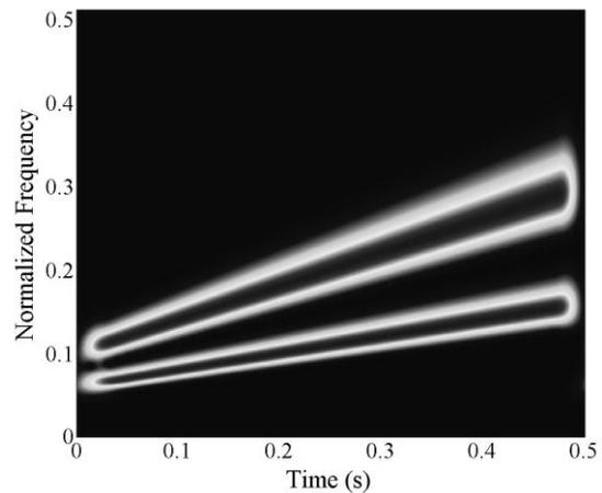
**Figure 2. The Generalized S-transform of the Chirp Signal**
