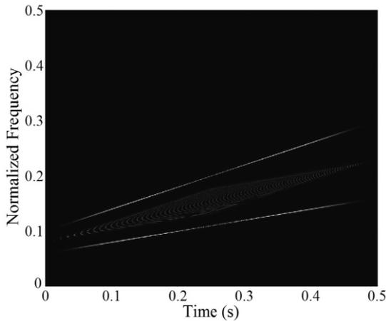
**Figure 1. The WVD of a Chirp signal**
