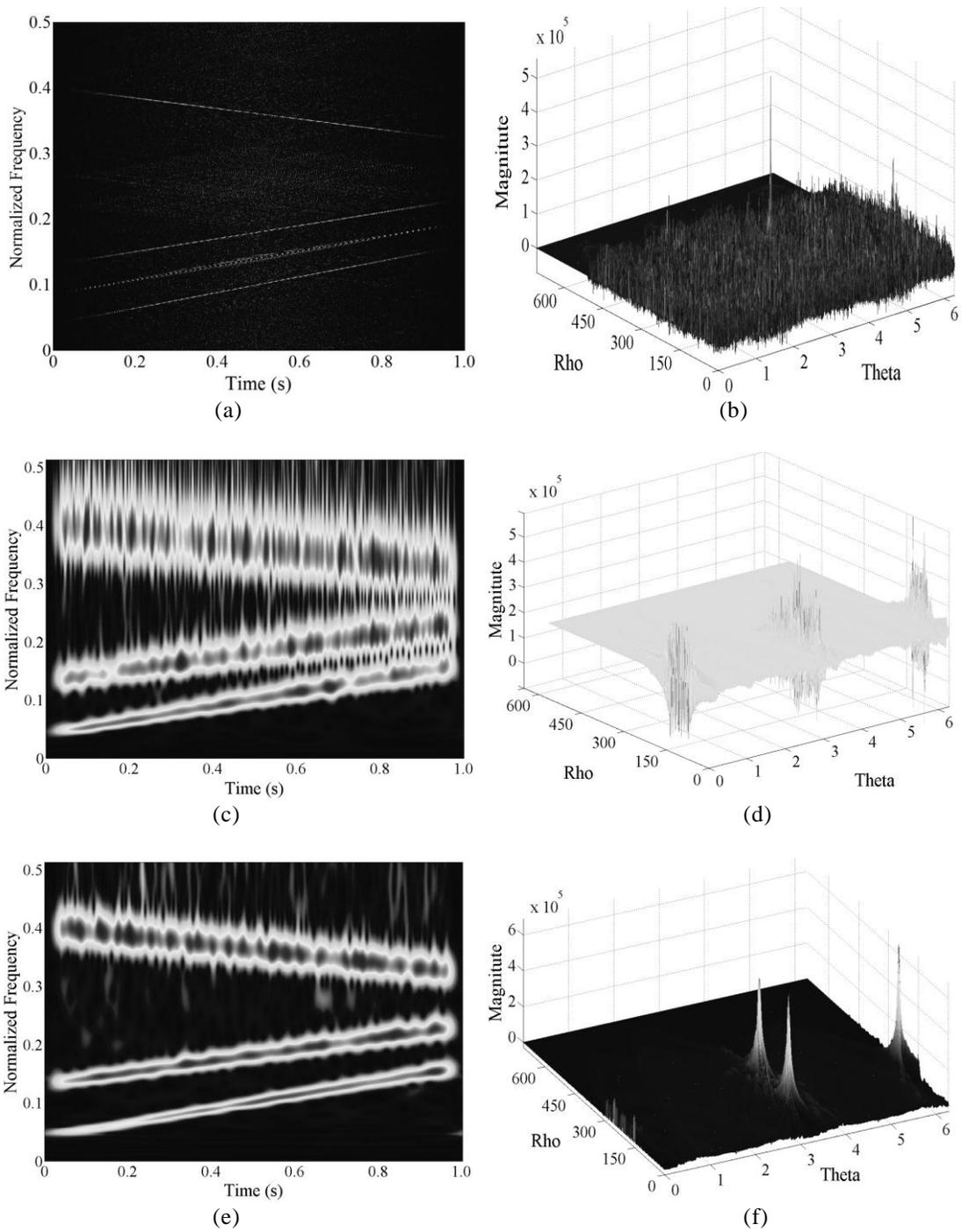
**Figure 4. Detection results of a three-component Chirp signal: (a) Signal detection result of WHT; (b) Parameters estimation result of WHT; (c) Signal detection result of S-Hough transform; (d) Parameters estimation result of S-Hough transform; (e) Signal detection result of generalized S-Hough transform; (f) The parameters estimation result of generalized S-transform and Hough transform**
