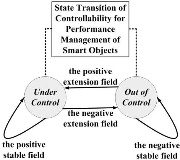
**Figure 3. State transition of controllability for performance management of smart objects with the use of the extension set**
