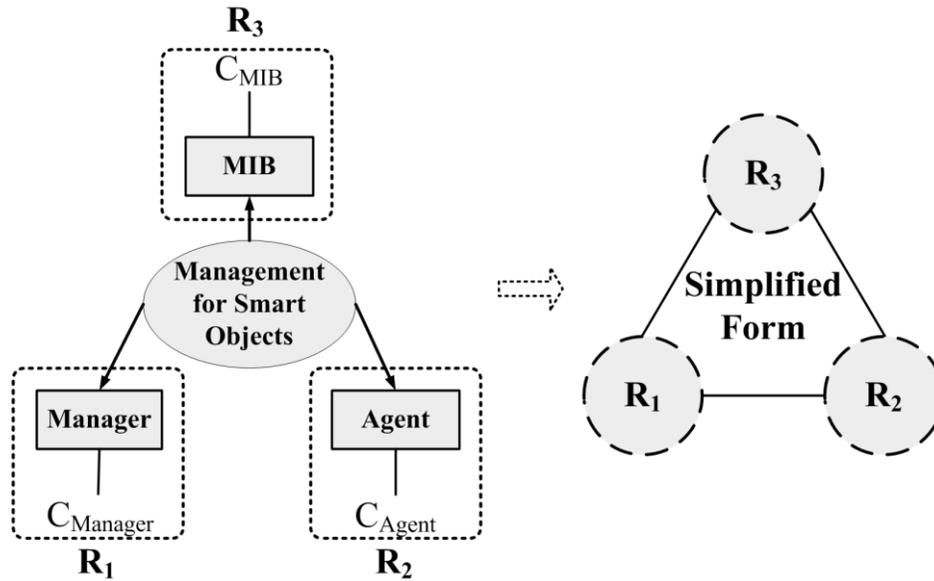
**Figure 2. A simplified form of the relationship of Manager, Agent and MIB for management of smart objects by relation-elements based on the extension model**
