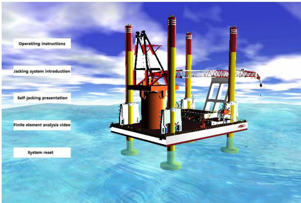
**Figure 5. The software interface of virtual prototyping of 800t jacking system of offshore platform**
