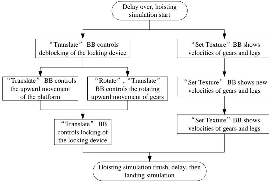
**Figure 10. The simulation process of hoisting**
