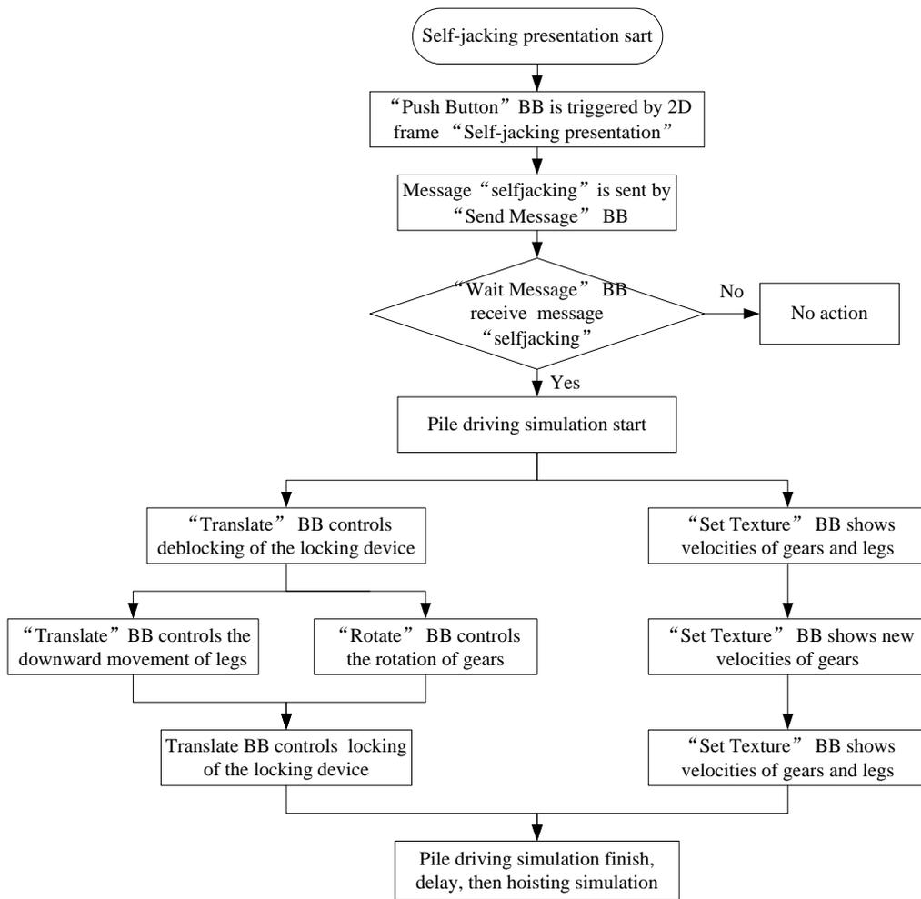
Figure 9. The simulation process of driving piles
