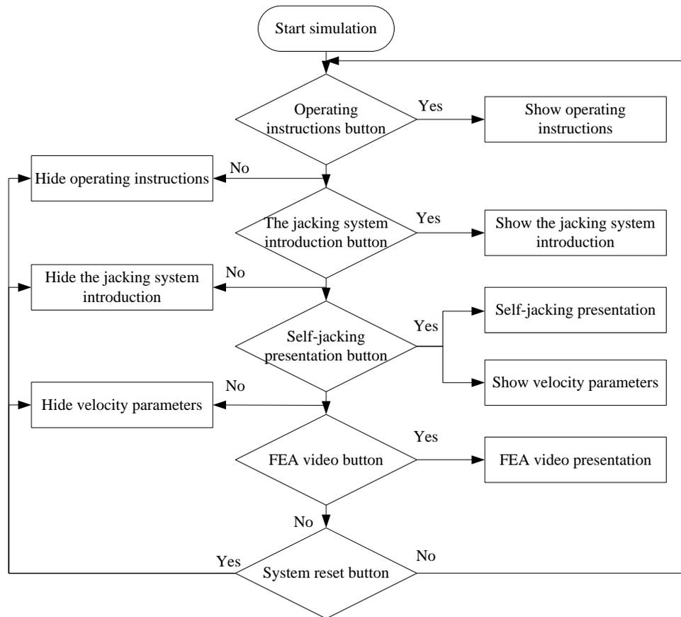
**Figure 6. The realization principle of the virtual prototyping for the jacking system**
