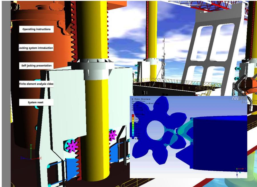
**Figure 14 Finite element simulation video of gears and legs**
