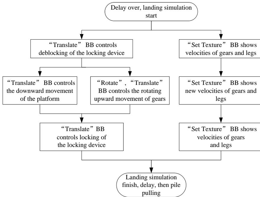
**Figure 11. The simulation process of landing**
