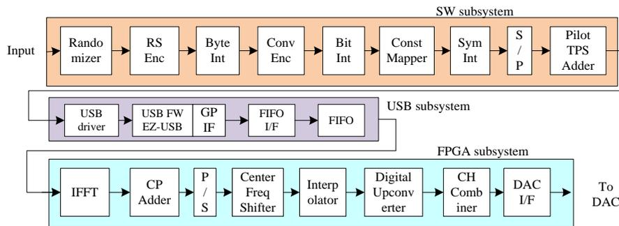
Fig. 1. DVB-T transmission system block diagram.
