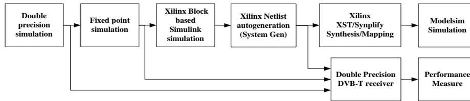
**Fig. 2.** Design flow of the DTV transmitter system using Matlab simulink and Xilinx block set.
