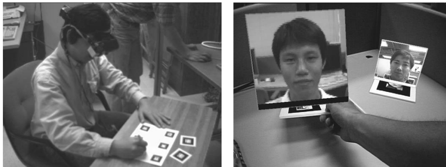
Figure 2. Marker based augmented reality system
