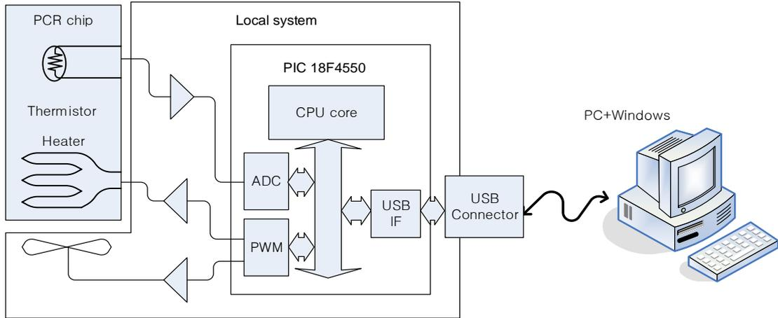
**Figure 1. PCR Chip and Its Control System**
