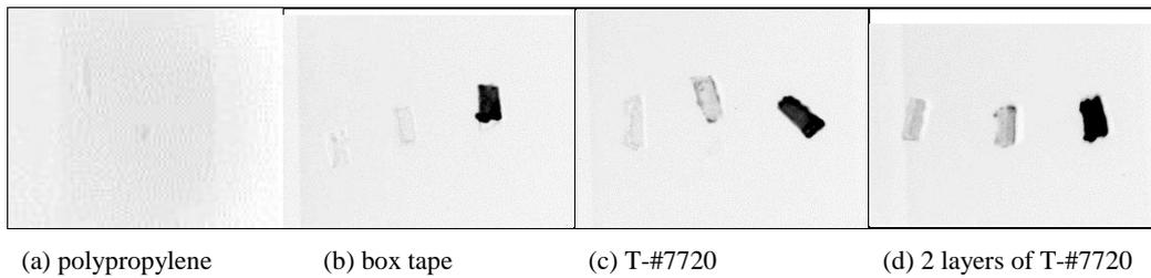
**Figure 3. Fluorescence Adsorption Test Images when BSA was not Added (The Leftmost Piece in the Image was not Immersed in the PCR Mix, and the Center Piece was Immersed for a While, and the Rightmost Piece was Submerged in the PCR Mix During the Whole PCR Process).**
