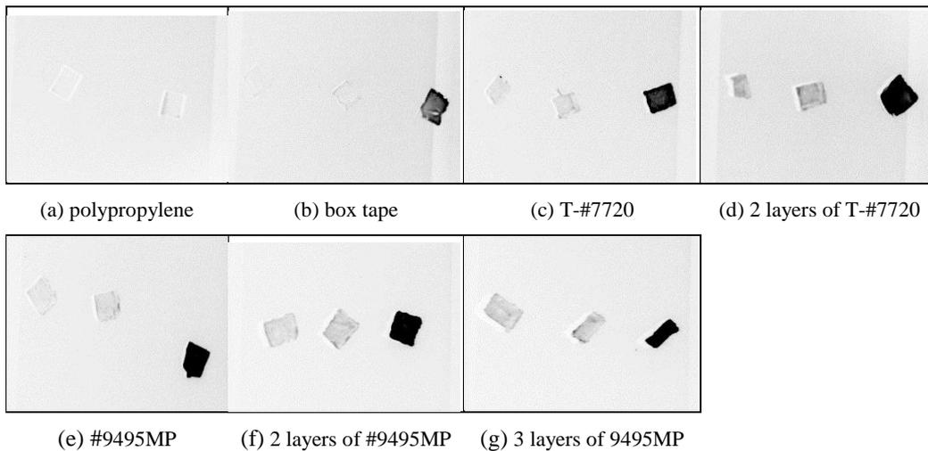
**Figure 4. Fluorescence Adsorption Test Images when BSA was Added (The Leftmost Piece in the Image was not Immersed in the PCR Mix, and the Center Piece was Immersed for a While, and the Rightmost Piece was Submerged in the PCR Mix During the Whole PCR Process)**
