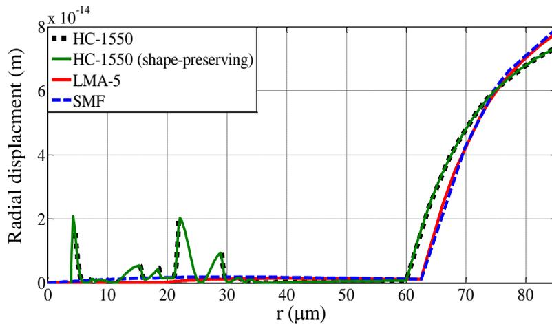
**Figure 3. Radial Displacement as a Function of Fiber Radius for (a) HC-1550, (b) LMA-5, and (c) SMF, for  $p = 5$  Pa,  $f = 10$  kHz**
