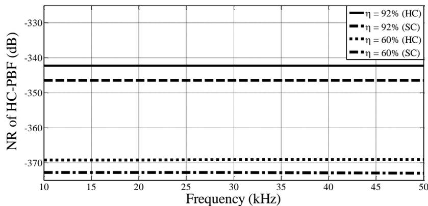
**Figure 6. NR of HC-PBF as a Function of the Acoustic Frequency for Different Air-Filling Ratios (HC) Indicates using the Same Structure with Hollow-core, while (SC) Indicates using the Same Structure with Solid-Core**
