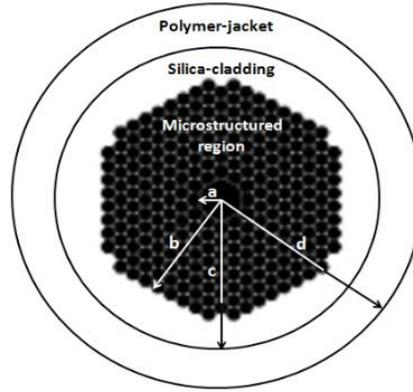
**Figure 1. General Cross-Section of a PCF with an Air/Solid Core, Honeycomb Air-Silica Inner Cladding, a Solid Silica Outer Cladding, and a Polymer Coating, where (a-d) Represent the Radius of Each Layer**
