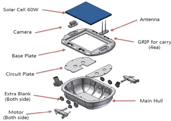
**Figure 6. Robot Platform Internal Structure**
