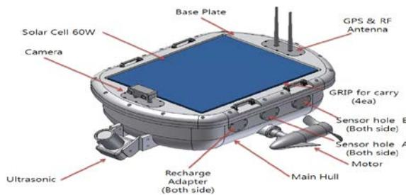
**Figure 5. Sensor Robot**
