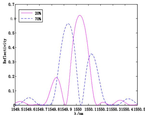
Figure 2. Reflection Spectra of FBG-FP at Different RH
