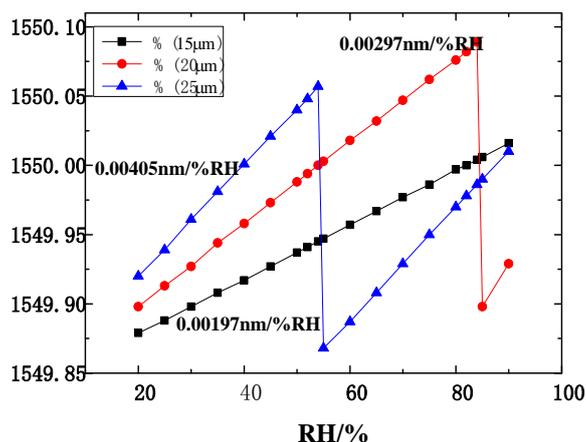
**Figure 7. Humidity Response under Different Thickness**
