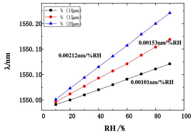
**Figure 5. Humidity Response under Different Thickness**
