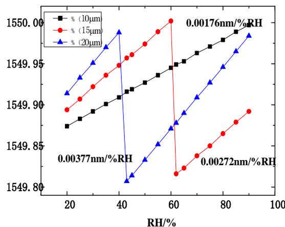
Figure 3. Humidity Response under Different Thickness
