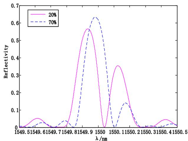
**Figure 6. Reflection Spectra of FP Cavity at Different RH**
