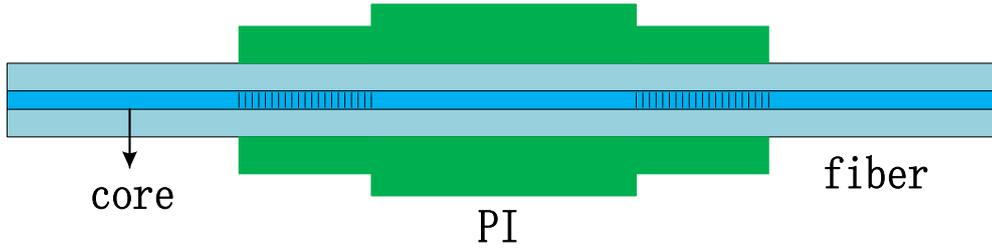
**Figure 1. Schematic of Grating F-P Cavity Coated with Polyimide**
