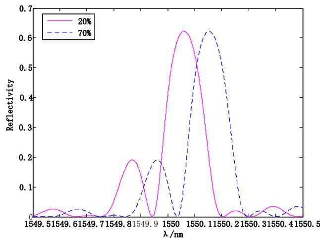
Figure 4. Reflection Spectra of FP Cavity at Different RH
