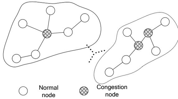
**Figure 2. Network Partition based on Congestion Nodes**
