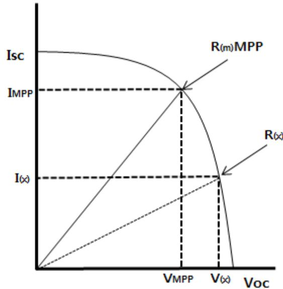
Figure 1. A MPP Graph of  $V_{OC}$  and  $I_{sc}$
