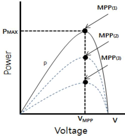
Figure 2. A MPP's Change Pursuant to the Power
