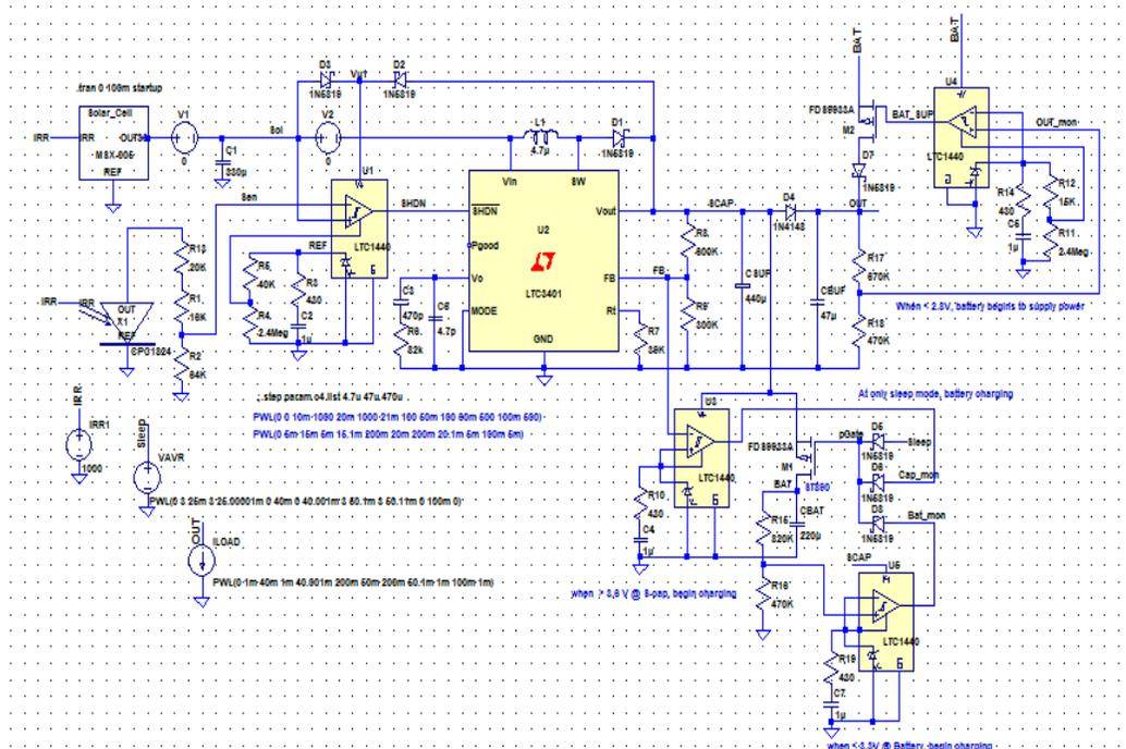
**Figure 13. A Simulation Circuit**
