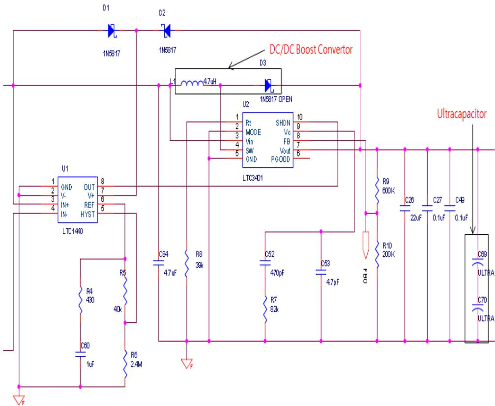
**Figure 4. A Comparator and a DC/DC Converter**
