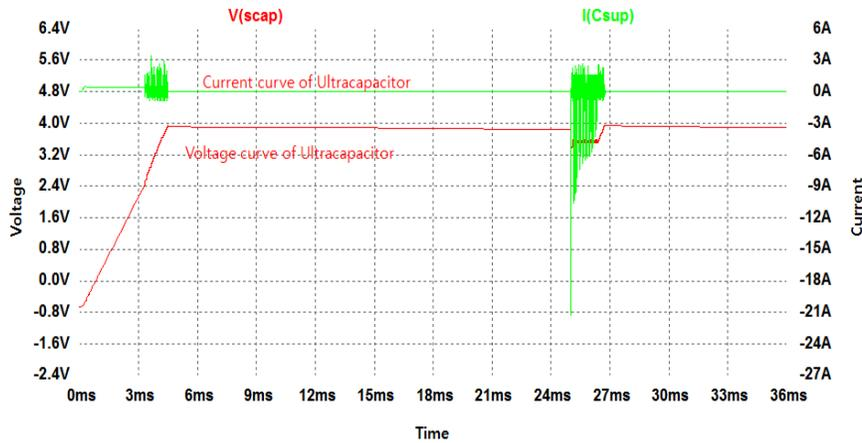
**Figure 15. A Voltage and a Current at the Ultra-capacitor Stage of the Circuit**
