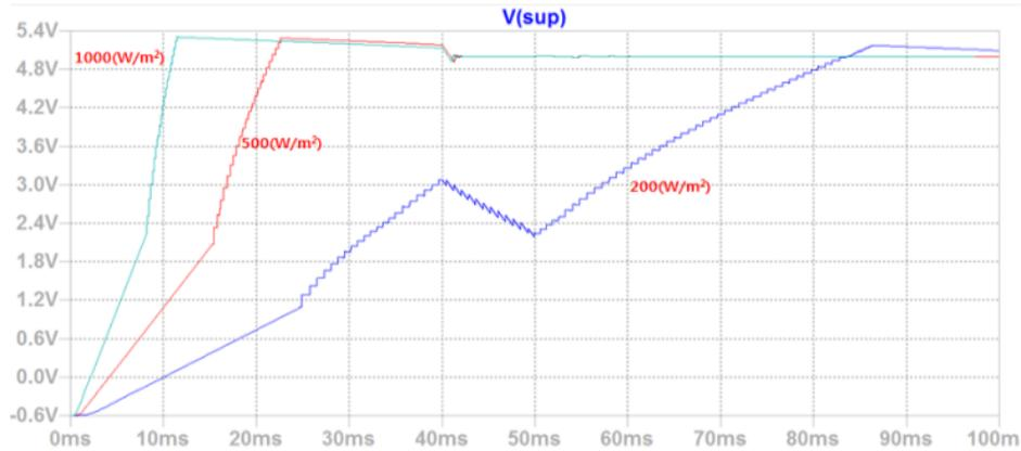
**Figure 12. A Simulation of Input Energy Intensity According to the Output Voltage**
