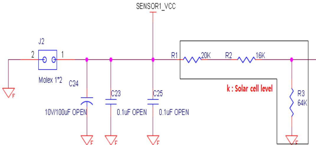
Figure 3. An Input Voltage Level
