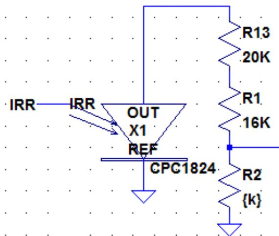
**Figure 5. A Simulation Circuit for the Input Voltage Level  $k$**
