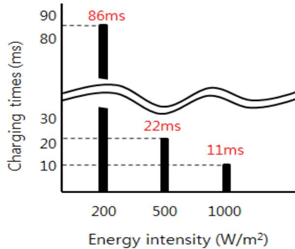
**Figure 10. An Input Energy Intensity According to the Ultra-capacitor Charging Time**
