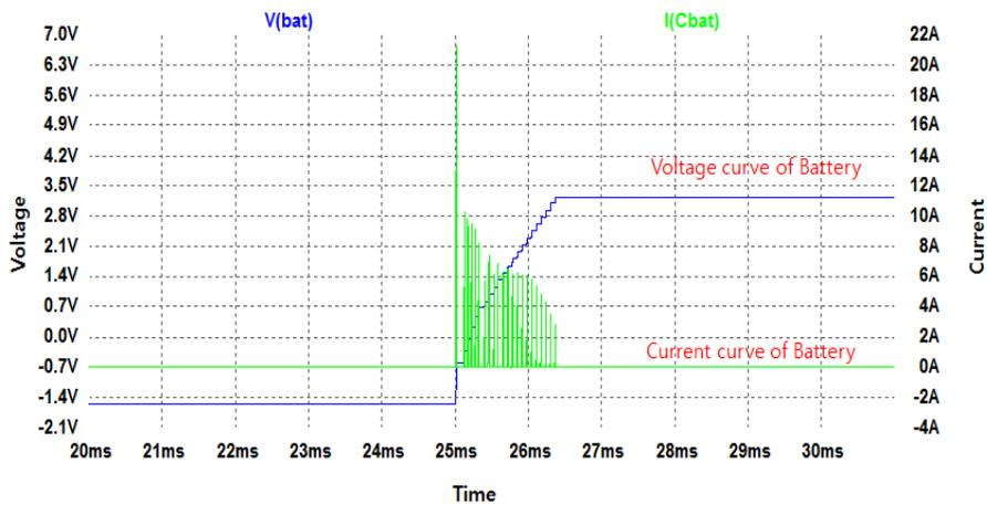
**Figure 16. A Voltage and a Current at the Battery Stage of Circuit**
