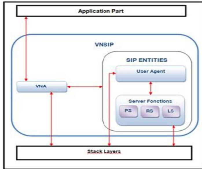
Figure 1. VNSIP Node Architecture
