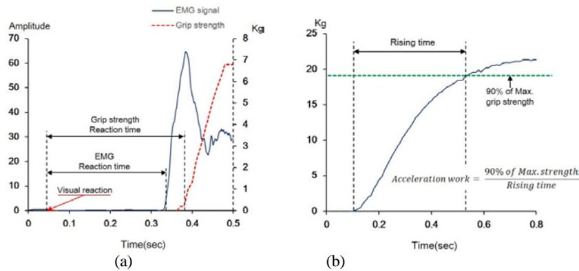
**Fig. 1.** (a) Changes in grip strength and EMG signals in agility exercise (b) Rising time and acceleration work in power exercise
