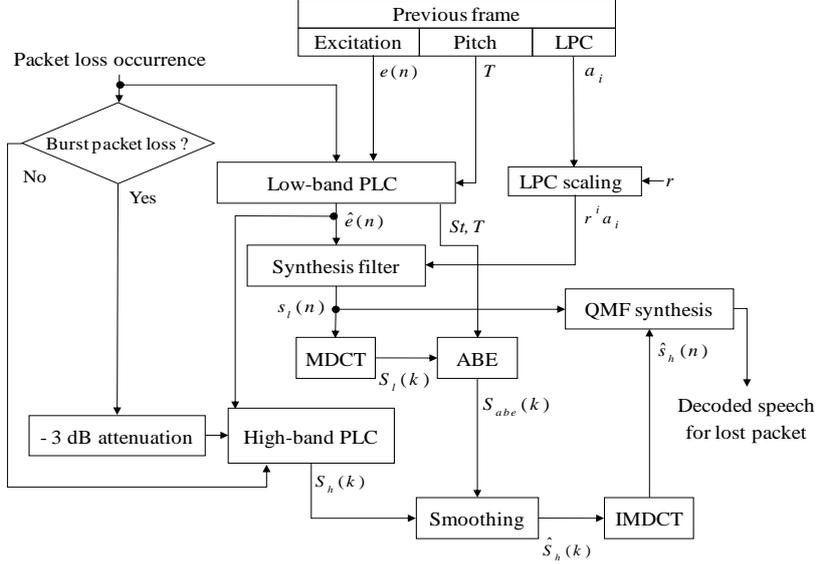
Fig. 1. Block diagram of the proposed ABE-based PLC algorithm.
