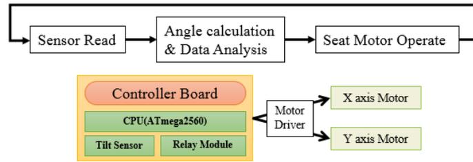
**Figure 3. System Operation Procedures for Balancing Seat**
