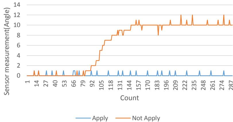
**Figure 12. Comparing the Tilt Sensor Value in Case Gyro Sensor is Applied and Not Applied**
