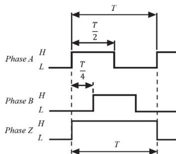
**Figure 5. Phases A, B, Z Using in the Incremental Encoder**
