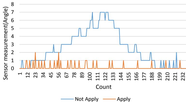
**Figure 11. The Output Result in Case Gyro Sensor is Applied and Not Applied**
