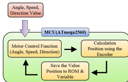
**Figure 6. The Motor Controller Operating**
