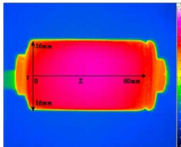
Fig. 1. The surface temperature distribution map after the 1200min charging is shown.
