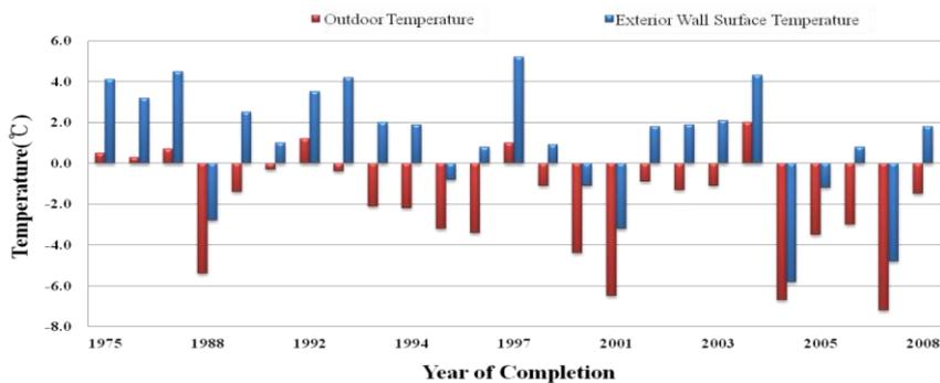
Fig. 2. Outdoor Temperature & Exterior Wall Surface Temperature Measurement Result
