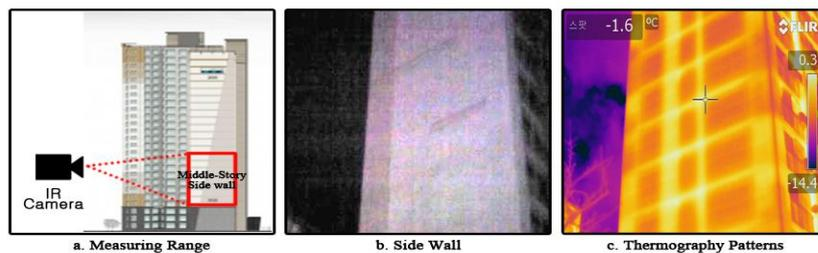
Fig. 1. Analysis Range and Surface Temperature Measurement
