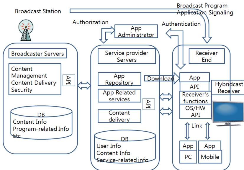
Fig. 1. The architecture of Hybridcast system
