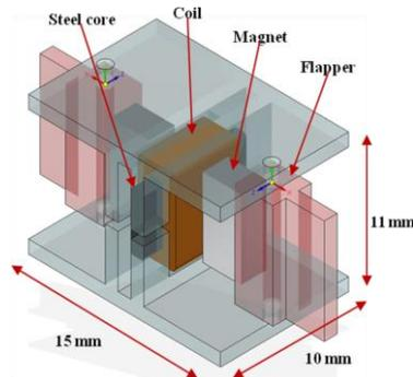
Fig. 1. Design of the moving magnet type voice coil actuator.
