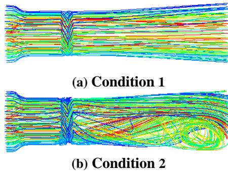
**Figure 9. Fluid trajectories in different working conditions**
