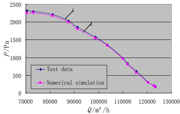
**Figure 11. The P-Q curves of test data and numerical simulation data**
