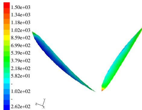
**Figure 6. Static pressure cloud map at the two impeller tips**
