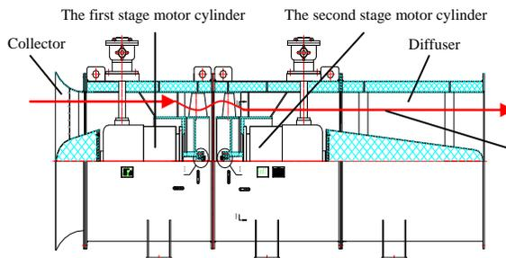
Figure 1. The structure of the counter-rotating fan
