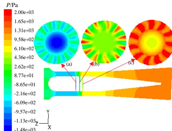
Figure 3. The static pressure distribution chart in axial section
