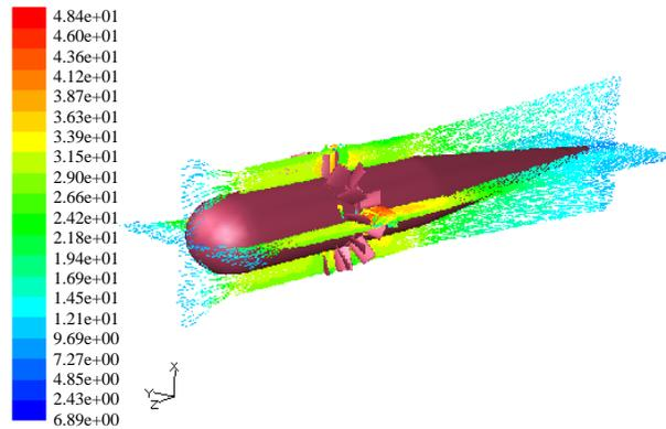
**Figure 7. Velocity vector in an axial cross**
