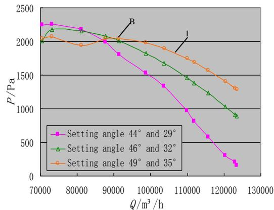
**Figure 12. The counter-rotating fan's P-Q curves in different blade setting angles**
