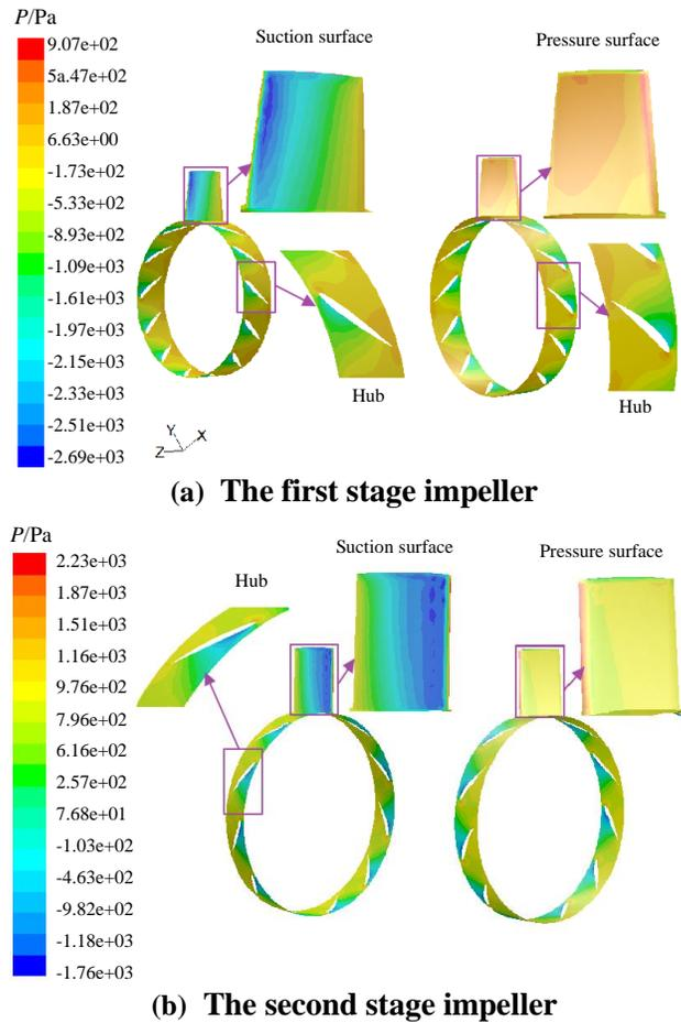
**Figure 5. The static pressure distribution in two-level impellers' root segments and blades**
