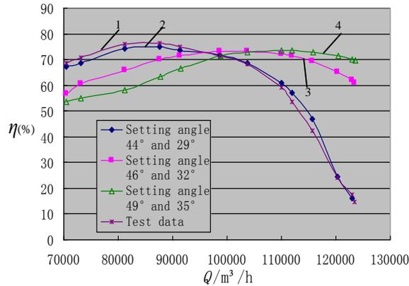
**Figure 13. The counter-rotating fan's efficiency curve in different blade setting angles**
