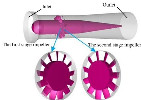
Figure 2. The global flow field model of the counter rotating fan
