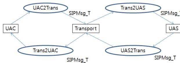
Fig. 3. The topmost level CPN model of SIP [1]
