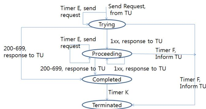
Fig. 2. SIP non-invite client transaction state machine
