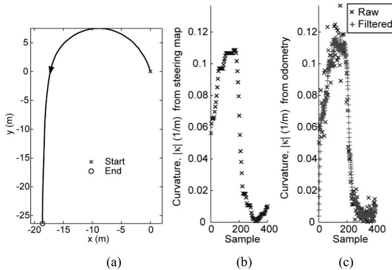
**Fig. 3.** Experimental results; (a) robot trajectory path, (b) curvature from the steering map, and (c) curvature from odometry.
