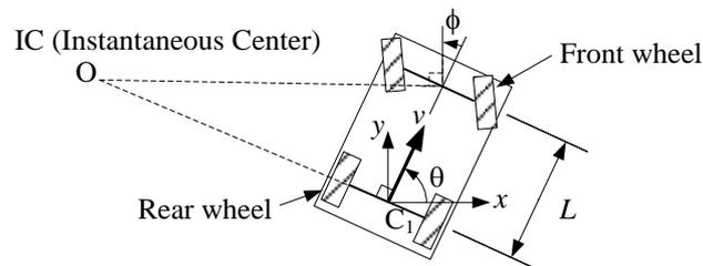
Fig. 2. Kinematics of a car-like robot.
