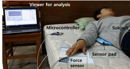
**Figure 1. System Configuration**
