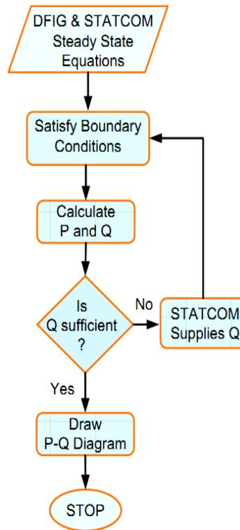
**Figure 5. Flowchart for Plotting PQ Diagram of DFIG-based WECS with STATCOM**
