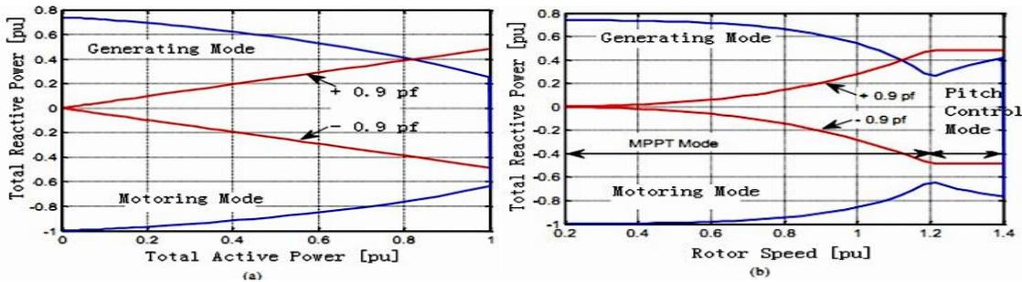
Figure 3. DFIG Steady State Reactive Power Capability Curves
