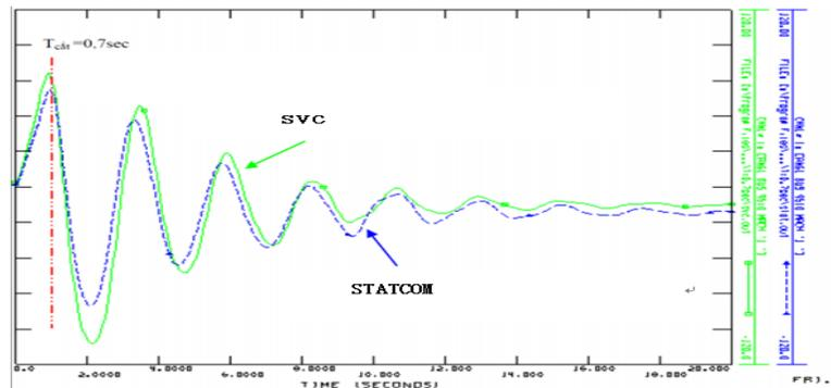
Figure 10. Phase Angle Oscillation of 1000MW Generating Set in Tra Vinh
