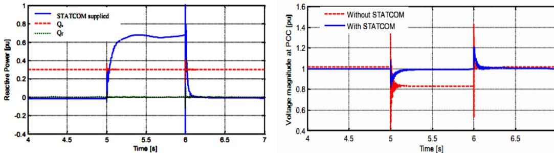
**Figure 9. The PCC Voltage at the DFIG Wind Turbine With and Without STATCOM during 18 % Symmetrical Voltage Sag**
