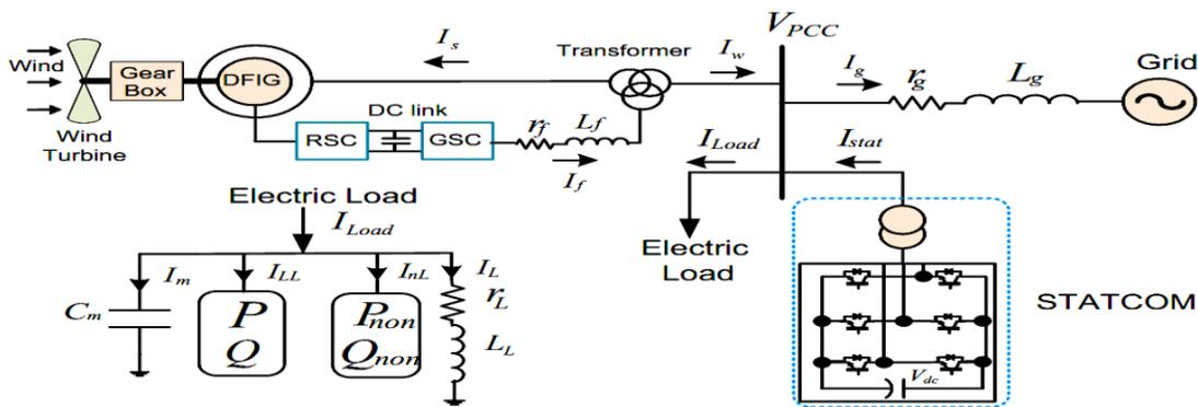
**Figure 7. Single Line Diagram of the Studied Power Network**
