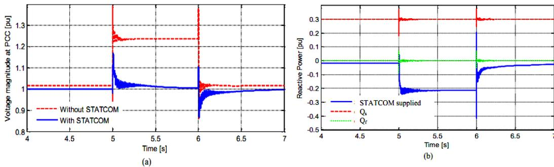
**Figure 8. The PCC Voltage at the DFIG Wind Turbine with and Without STATCOM During 22% Symmetrical Voltage Swell**
