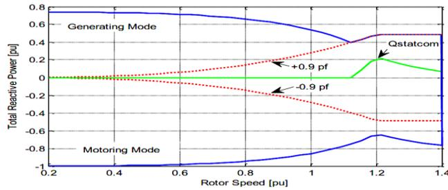
**Figure 6. Reactive Power Capability Diagram of Overall DFIG-based WECS with Statcom at Various Rotor Speeds**
