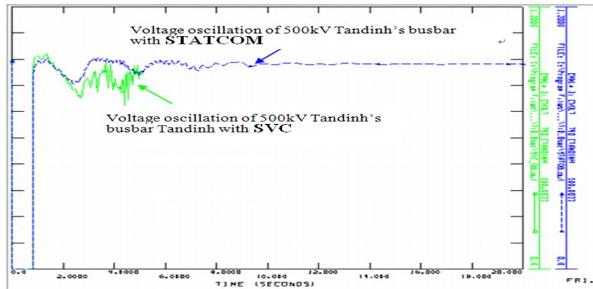
Figure 11. Voltage Oscillation of 500kV Tandinh's bus bar
