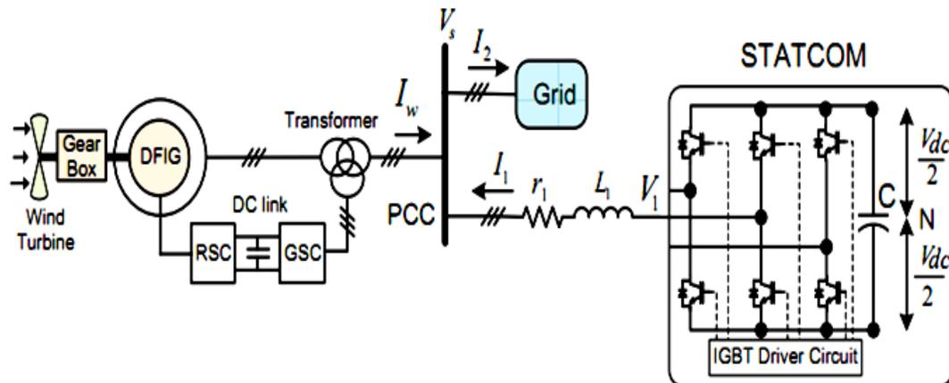
Figure 4. STATCOM Connected to DFIG-based WECS at PCC
