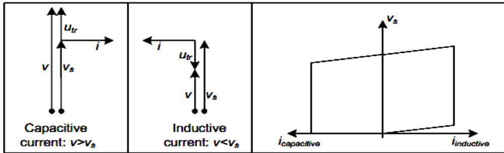
**Figure 2. Operating Principle and Operation Area of STATCOM**
