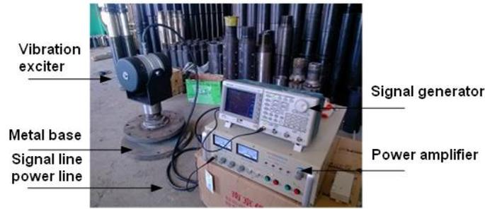
**Figure 6. Exciter and Signal Transmitting Devices**
