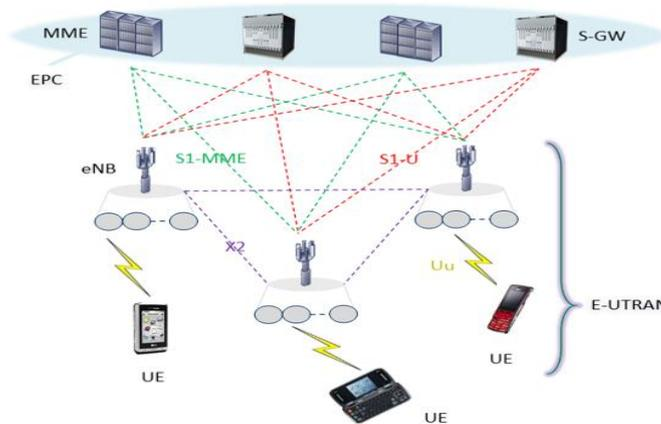
Fig. 3. 3GPP Overall architecture
