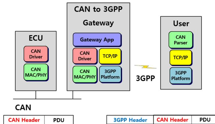
Fig. 5. CAN over 3GPP Gateway Concept
