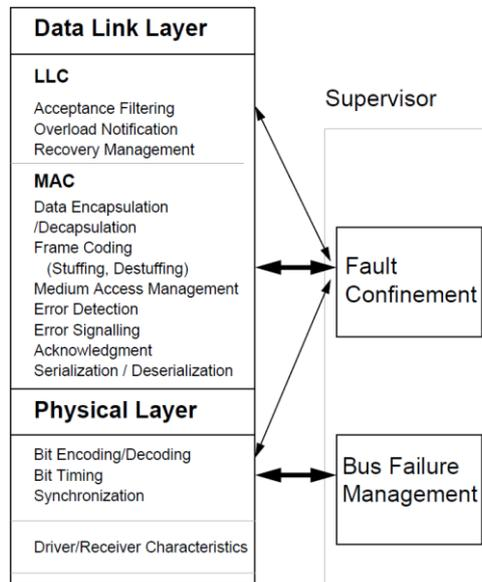
**Fig. 2.** Layered Architecture of CAN according to the OSI Reference Model [1]
