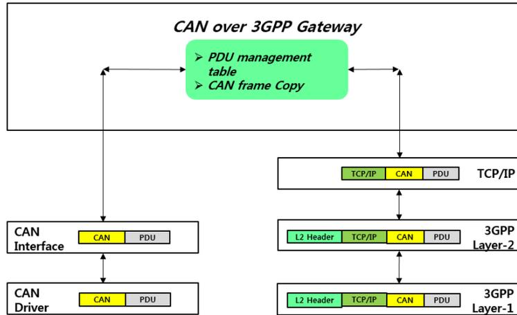
Fig. 6. The flow diagram of the CAN over 3GPP Gateway
