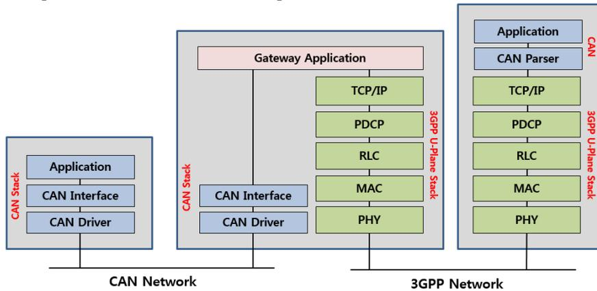
Fig. 7. Protocol Stack of the CAN over 3GPP gateway
