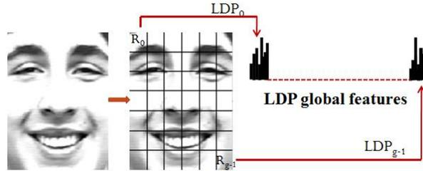
**Figure 4. Expression image is divided into small regions from which LDP histograms are extracted histograms are extracted and concatenated into LDP global features**
