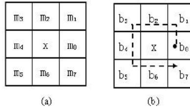
**Figure 2. (a) Eight directional edge response positions; (b) LDP binary bit positions**
