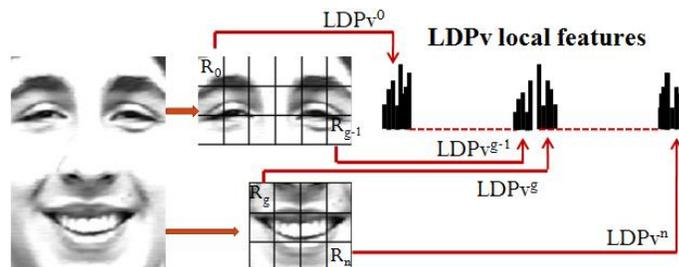
**Figure 5. LDPv histograms are extracted from the regions of eyes and mouth and concatenated into LDPv local features**
