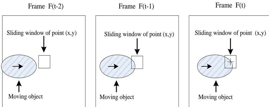
**Figure 2. Motion Detection**
