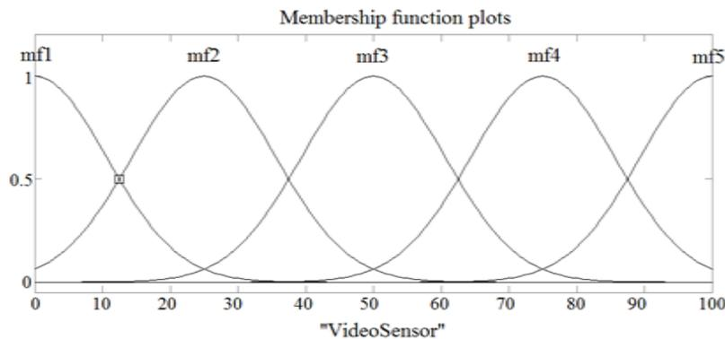
Figure 5. Member Functions of “Video sensor”.
