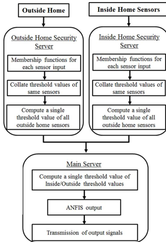
**Figure 1. Security inference structure using ANFIS**
