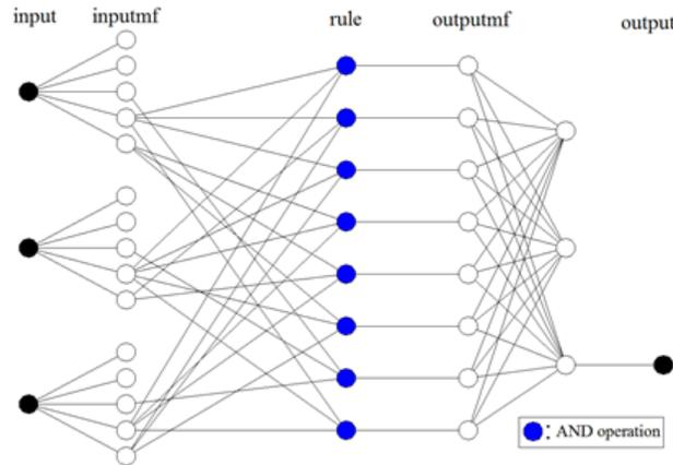
**Figure 6. ANFIS structure for sample scenario**
