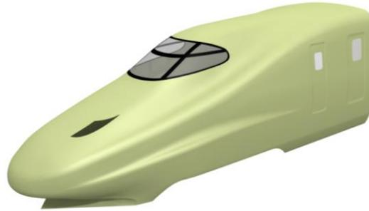
**Figure 10. Surface Model of the Driver Cab**
